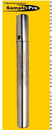
The SamplePro Portable MicroPurge Pump uses a quickchange, one-piece bladder design. Compressed gas squeezes the outside of the bladder to force liquid out of the pump; there is no gas contact with the pumped water inside the bladder.
